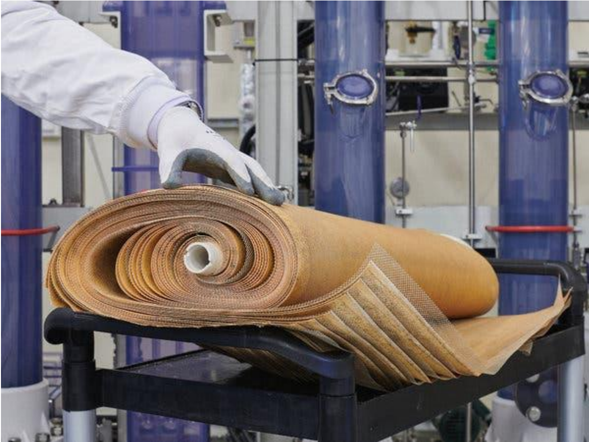
A sheaf of reverse-osmosis membranes, unfurled to show the layers that separate salt from water.
